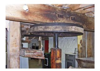
The shaft from one of the planet wheels on the floor below turns the belt wheel.
