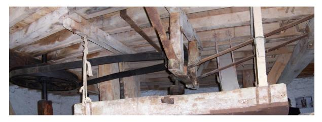
Not all the power in the mill is transmitted by gears. Here, below the millstones a chute delivers flour to a sieve, and this is shaken by a mechanism which gets its power from a belt connecting the wheel on the left to a wheel directly over the sieve.
