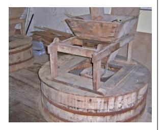
The shaft of the planet gear passes up through the floor and turns the top stone of a pair of mill stones. You cannot see the actual stones in this photo, because they are hidden inside this wooden case. Grain from the floor above pours into the wooden hopper at the top of the case, and is shaken into the opening in the top of the upper millstone. It is ground into flour between the stones, and goes through a chute to the floor below, where it is sifted and bagged.
